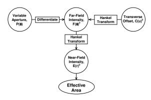
Figure 1. Relations between the techniques used to measure the effective area.
