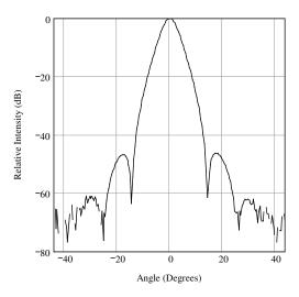
Figure 2. Example of a measured far-field intensity distribution including side-lobes. Matched cladding fibre at 1551 nm.
