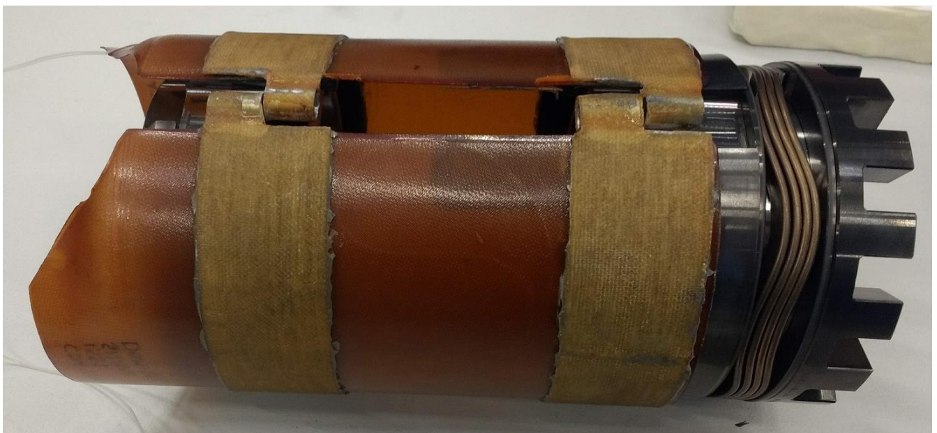
Figure 6: Axle sensor prototype, including clamping mechanism
