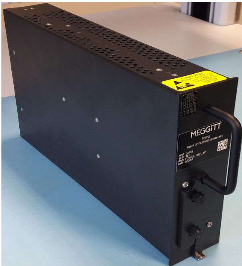
Figure 2: FOPU prototype- External view – ARINC 600 2MCU rackable avionic unit
