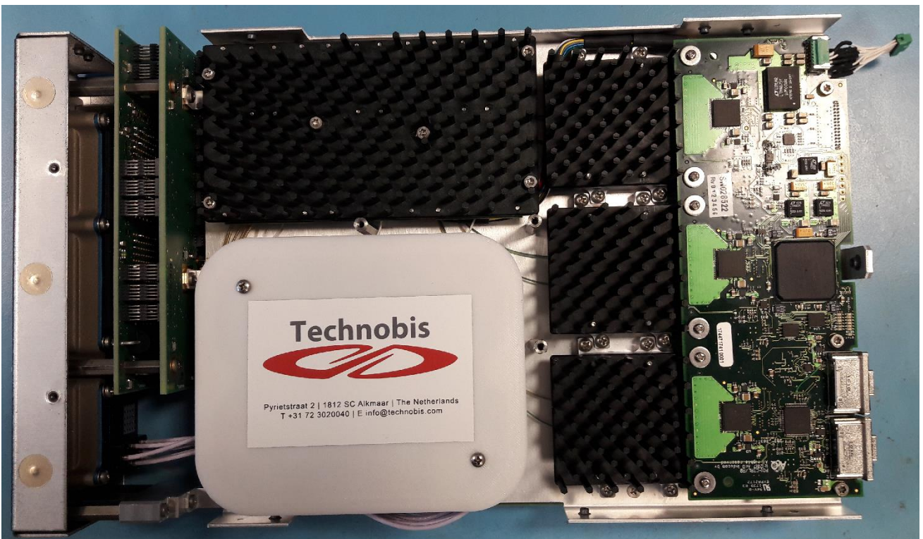
Figure 4: FOPU prototype - Optical part – 6-channel FBG interrogator fitted with heat sinks
