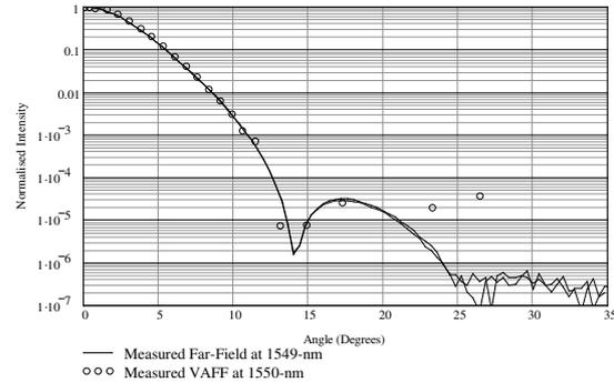
**Figure 3. DFF and VAFF measurements of the far-field distribution from an attenuation-flattened fibre.**
