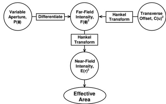
Figure 1. Relations between the techniques used to measure the effective area.
