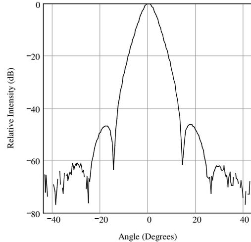
**Figure 2. Example of a measured far-field intensity distribution including side-lobes. Matched cladding fibre at 1551 nm.**
