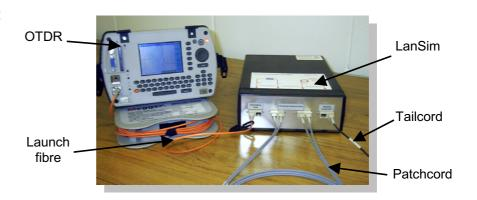
The LanSim LS-1 simulates a typical Local Area Network data link. It includes 15m of horizontal cabling with two different quality splices, and 50m of vertical cabling with a controlled duct restriction.
