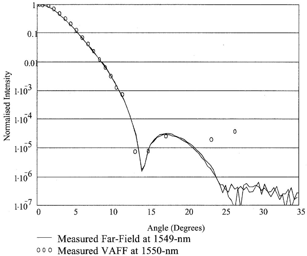
**Figure 3 DFF and VAFF measurements of the far-field distribution from an AllWave® fibre.**
